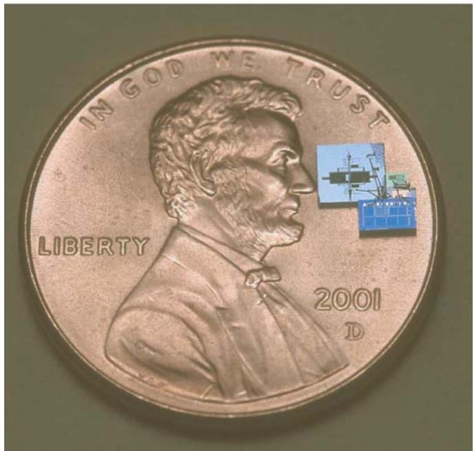
▲ **Figure 5-12** Smart dust. The visions for smart dust presume that it will be relatively undetectable by the human eye. Current research efforts have dramatically brought down the size of the dust. (Berkeley)
